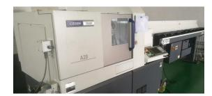
Many of our CNC lathes are equipped with automatic bar feeders, which allows us to machine larger batch quantities unattended and produce high volume machining with low labour inputs.
