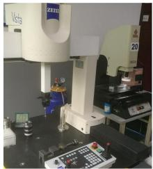
By employing digital calibration and measurement techniques (2 & 3 dimensional image detector e.g. CMM Zeiss), our full-time quality assurance department inspects at first-off, intermediate stages during production and final inspection to ensure products meet the required specifications and tolerances.
